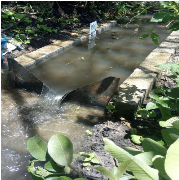
Figure 3: Field measurement of irrigation water using V-notch
