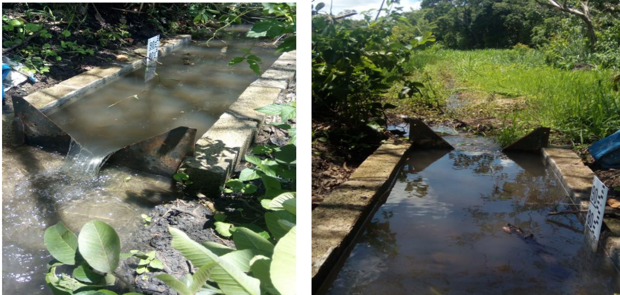
Figure 3: Field measurement of irrigation water using V-notch
