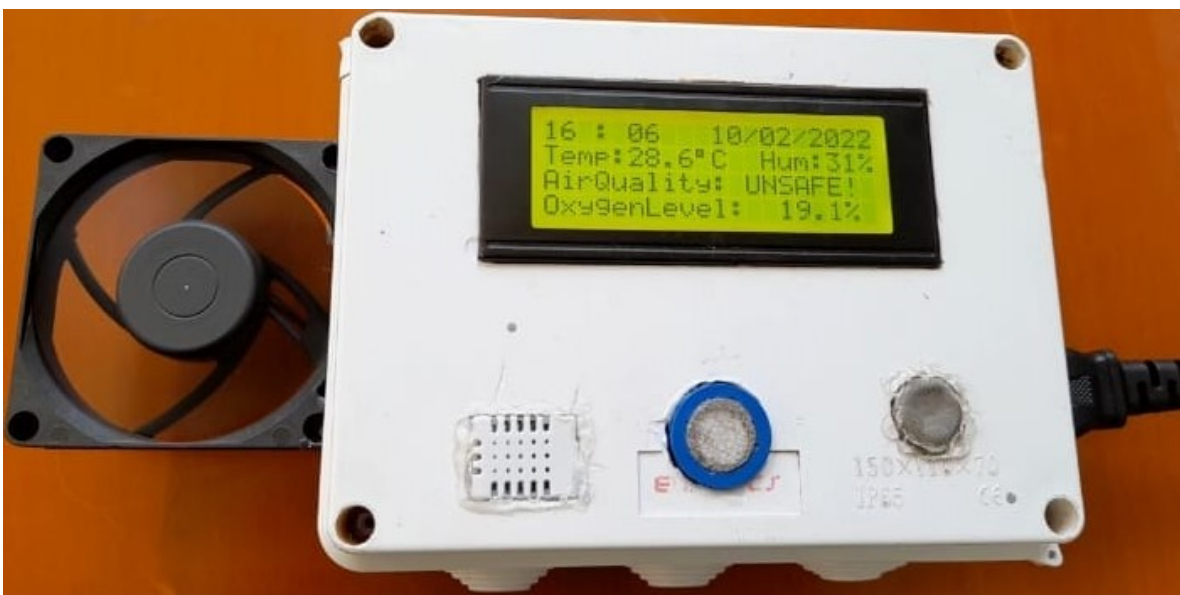
Figure 27: System displaying oxygen, air quality and temperature levels in unsafe mode
