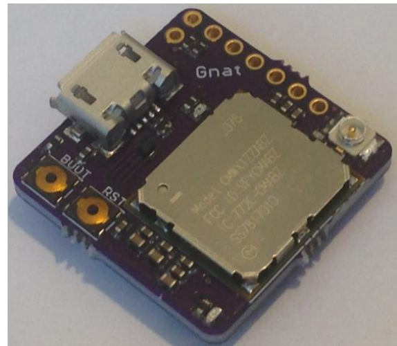
Fig. 3. CMWX1ZZABZ LoRa Module used for Data Transmission between Smart Meter units and Local Monitoring Centre.
