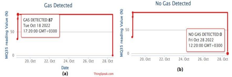
Fig. 13. Gas condition results around the boiler (a) Gas detected (b) No gas detected.
