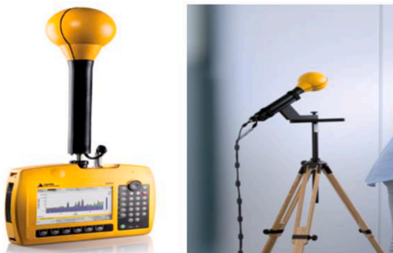
Fig. 3. Narda 3006 SRM with probe and wooden tripod stand.
