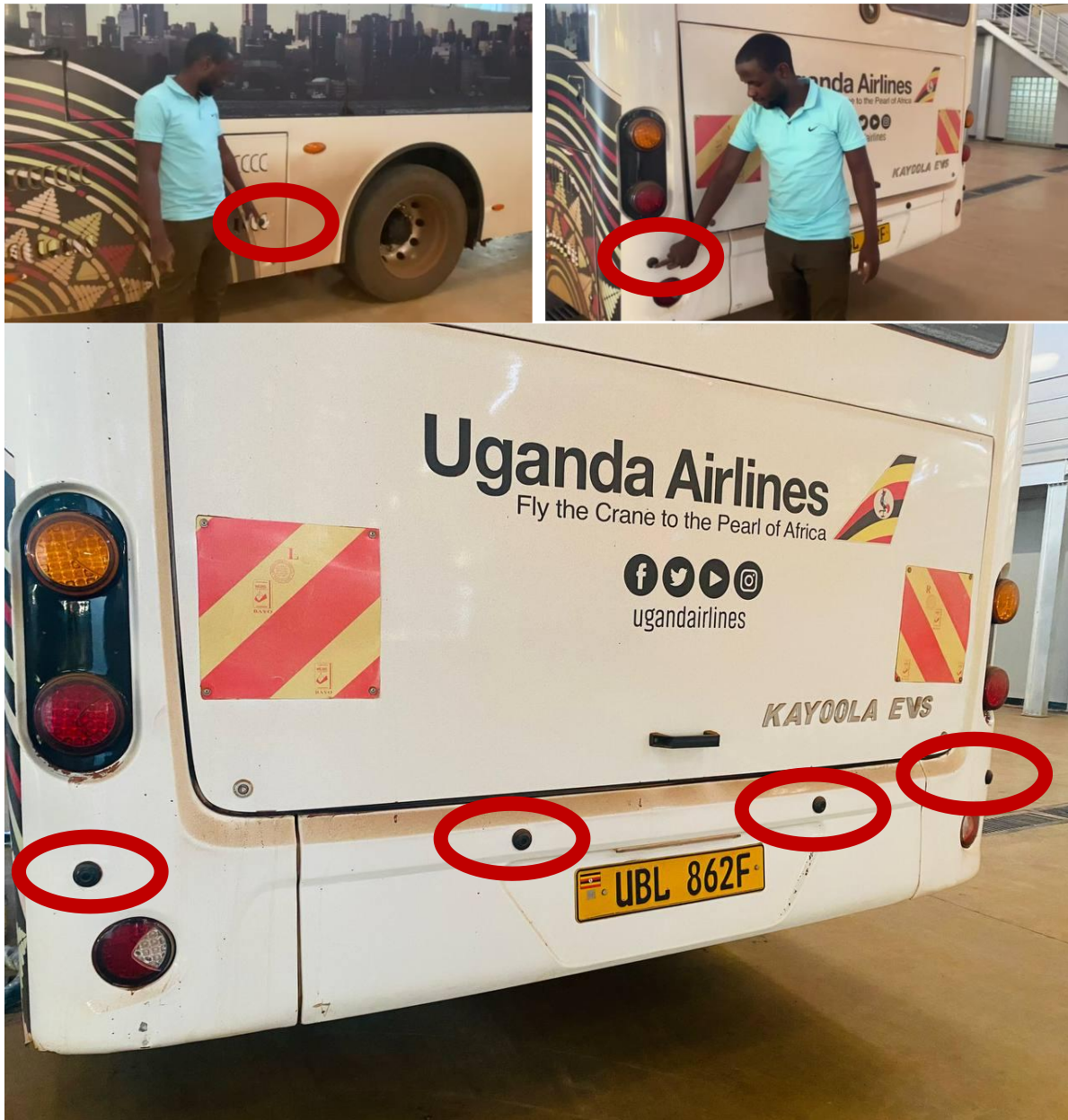
Figure 25: Integration of proximity sensors
