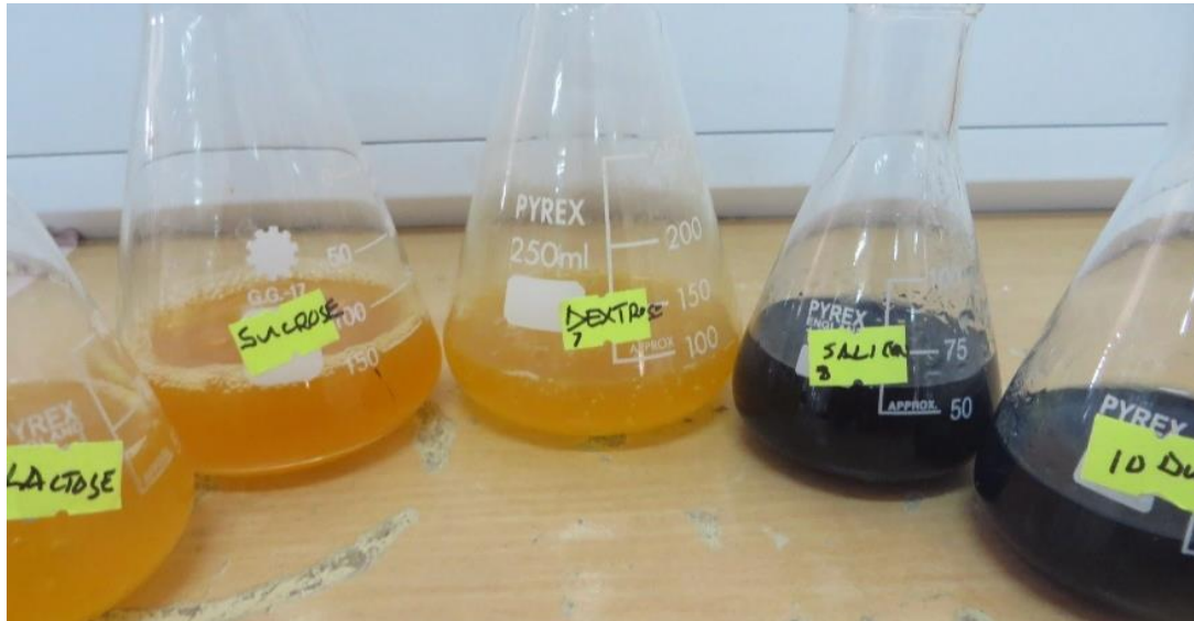
Figure 10: Utilization of the basic carbon sources as indicated by a colour change
